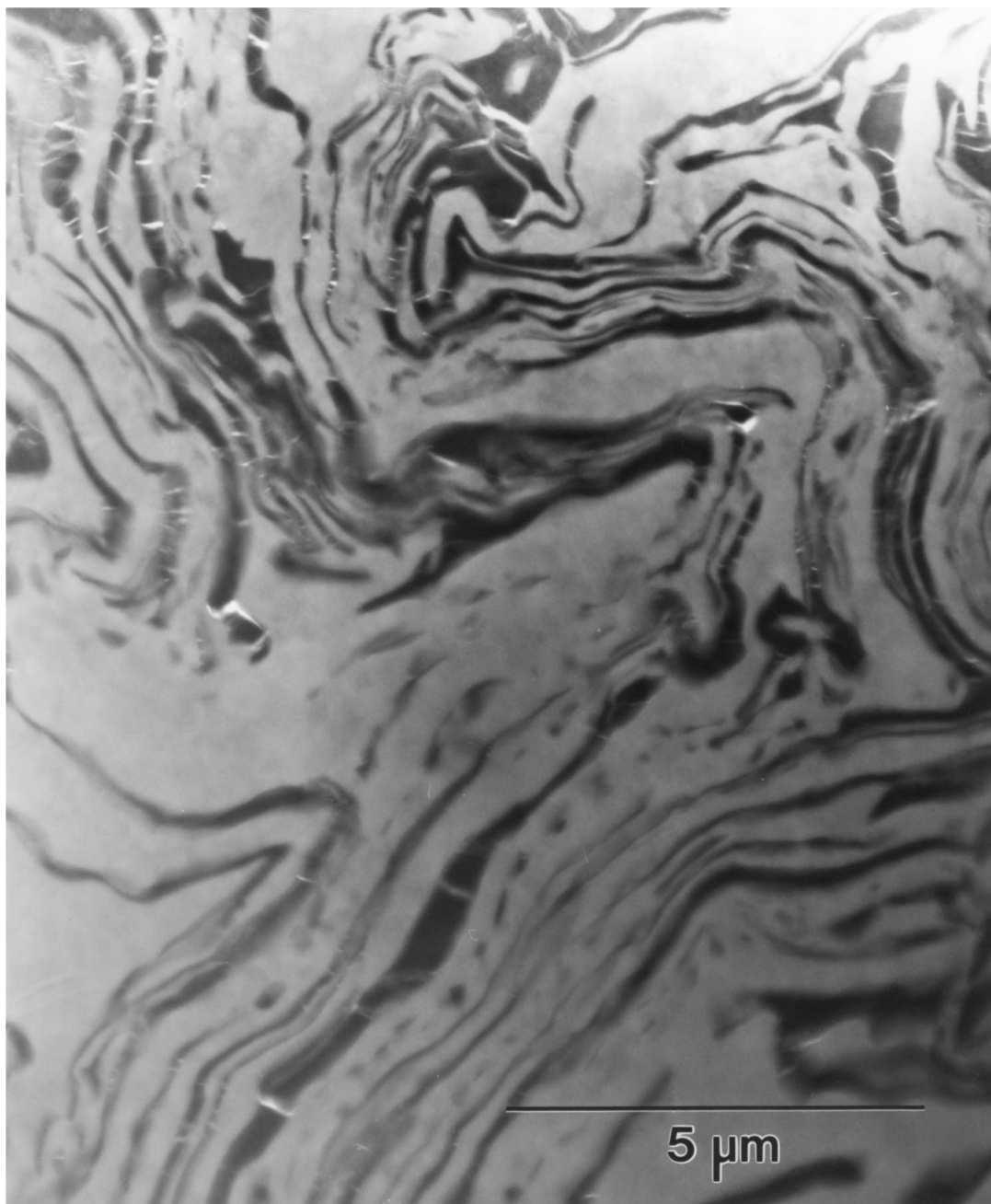
Figure 2 TEM micrograph of Ti-20Y axisymmetrically deformed to \eta = 5.03 . The imaging contrast in this micrograph renders the Y phase dark gray and the Ti matrix light gray. This transverse section of the specimen shows a point view of the rod axis and a true length view of the rod diameter.
