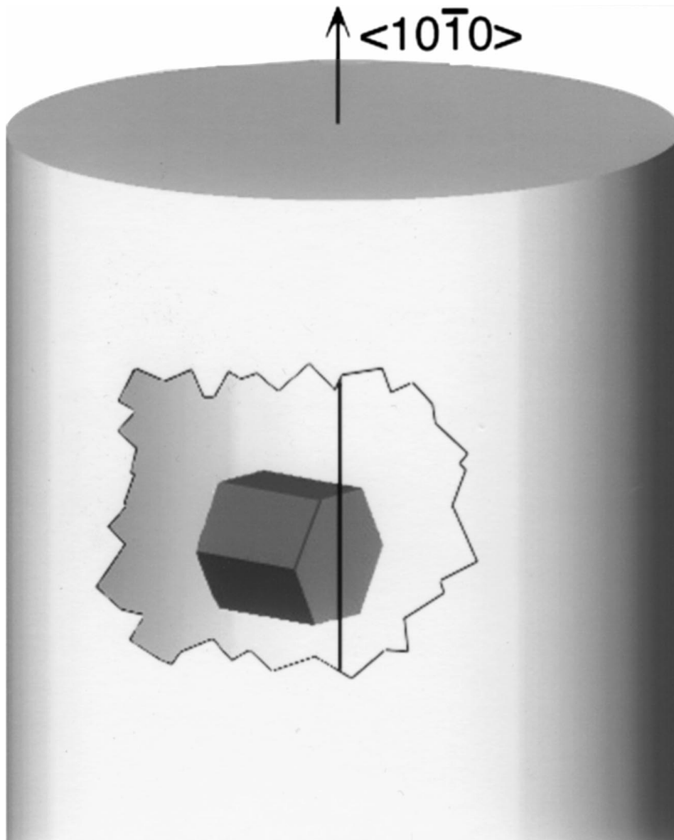
Figure 8 Depiction of an HCP unit cell oriented with the \langle 10\bar{1}0 \rangle direction parallel to the rod axis of an axisymmetrically deformed specimen.
